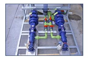
The extremely "wetted" polymer is hydraulically transferred to the mixing/ageing tank where it is stirred by a slow speed stirrer and allowed to age. After the required ageing time, prepared polymer is pumped or gravity fed to the storage/dosing tank and a new batch is commenced.
